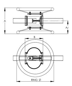
Cast of a lightweight and corrosion-resistant aluminum alloy, the economical type EHV WEC makes a permanent and reliable connection between tubes and offers protection for equipment bushings, switch gear, and insulators by compensating for expansion and contraction due to temperature variations.
